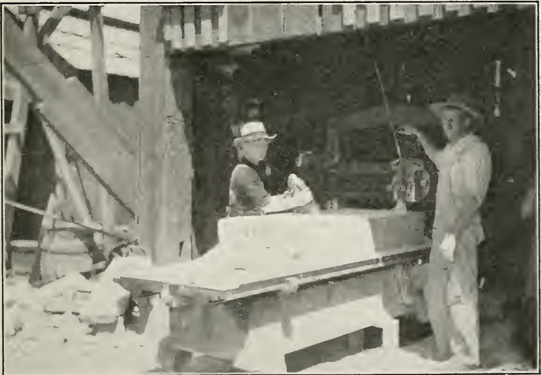
ILL. No. 3. VIEW OF STONE PLANER, BLY BROS.' STONE COMPANY, LOS ANGELES.
