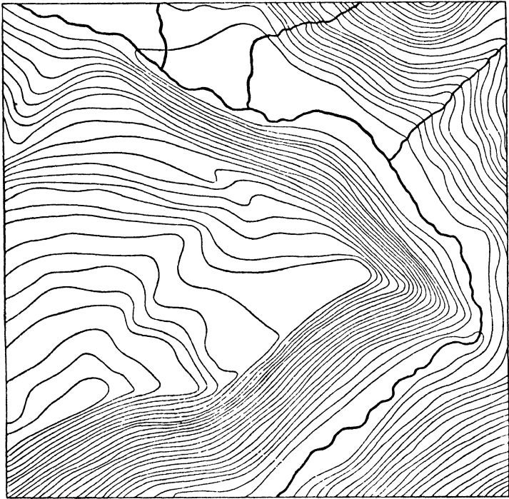
FIG. 18.—Map to show a valley worn into a hill-mass. The vertical interval between the contour lines is 100 feet. The horizontal scale is an inch to a mile.
